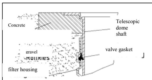
**Please note:** If the soft soap dries, the telescope can only move with great difficulty and there is a risk that the seal will slip out of the groove. Before filling, you must check that the seal is sitting correctly.
