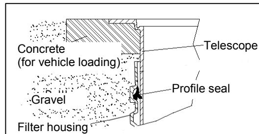
**Caution:** If the soft soap dries, the telescope becomes difficult to move and there is a risk that the seal may slip out of the seal groove. Before backfilling, the seal must be checked for a correct fit. The telescope must be sufficiently lined so that forces can under no circumstances be transferred to the housing.
